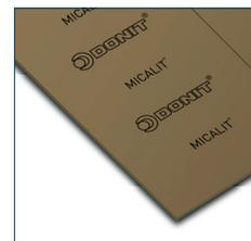
MICALIT<sup>®</sup> F contains a high percentage of phlogopite mica flakes, impregnated with a silicone binder. It has excellent thermal and good chemical properties, making it suitable for high temperature applications in the automotive and steel industry for exhaust systems, gas turbines, oil and gas burners, furnaces and ovens. It also offers good dielectric and low thermal conductivity properties.
